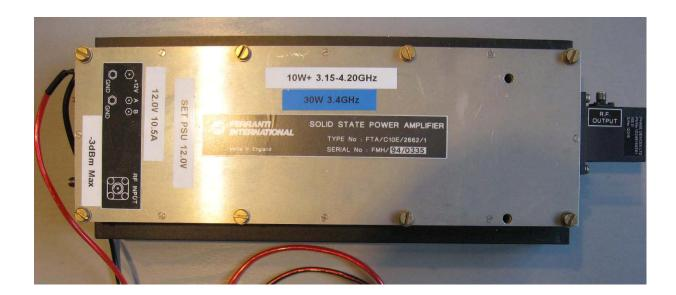
Using the parts shown a competitive (30W output, 0.85dB NF) 3400 MHz transverter was built for a cost around £150.
